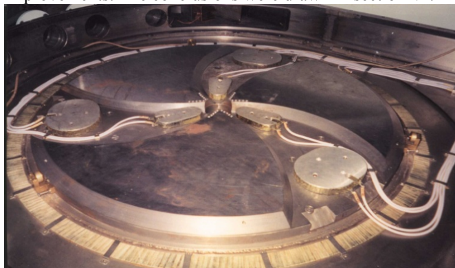
Fig. 1 Location of harmonic coils inside the chamber
